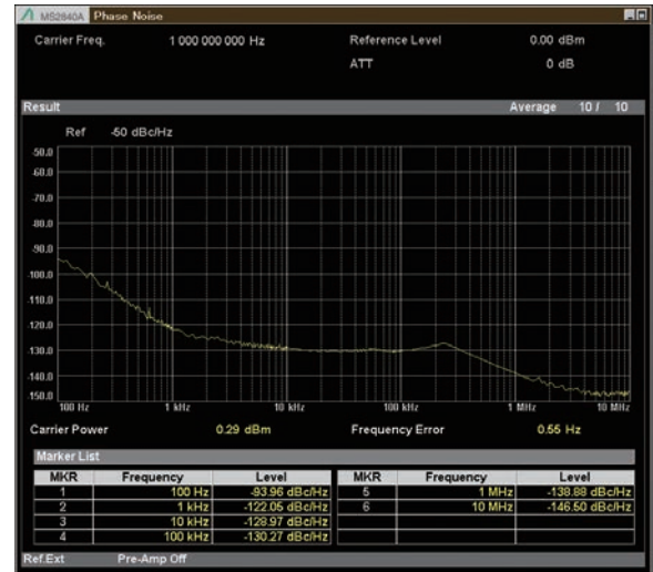
Phase Noise Measurement Low Phase Noise Performance MS2840A-066 Off 1 GHz Measurement Frequency, Preamp Off
